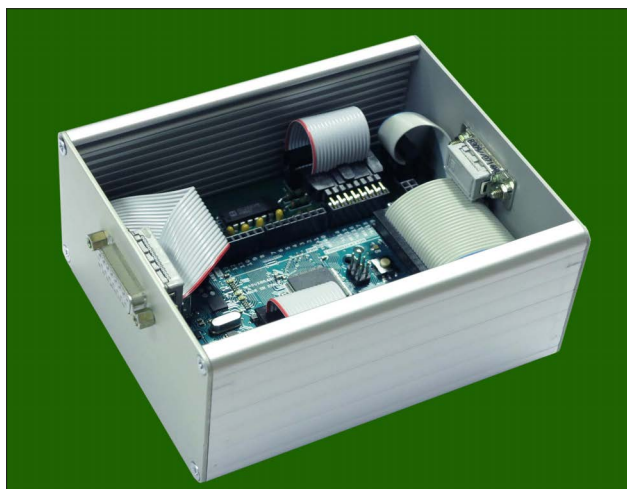
AVS47-Serial/USB-W Unit measures 130x105x60 mm and gets power from the +12V Mains Adapter.
