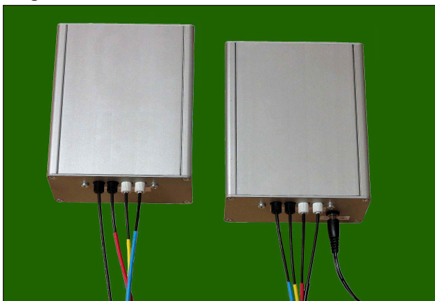
Both AVS47-Serial/USB-F units measure 130x105x60 mm. Box1 is powered by the resistance bridge and Box2 gets power from a +12V wall adapter.
