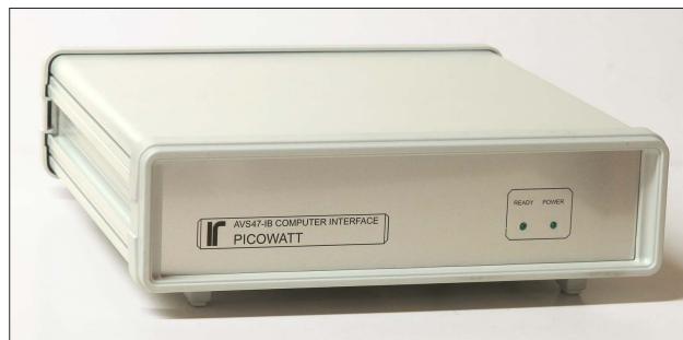
The AVS47-IB is a protocol converter between GPIB (IEEE-488) and Picobus. It is the heart of the "GPIB-Picobus" interface. Only limited availability.
